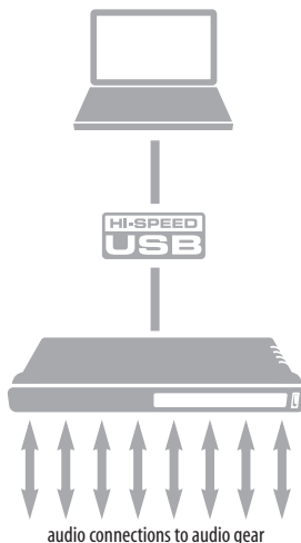
Figure 5-1: Using your MOTU AVB device as an audio interface.
