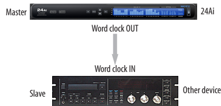
Figure 4-8: Slaving another digital audio device to your MOTU device (a 24Ai in this example) via word clock. For the 24Ai clock source, choose any source besides word clock, as it is not advisable to chain word clock.
